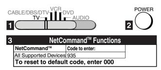
**Figure 1.** Programming the remote to control your Net-Command™ A/V devices.
